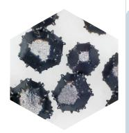
**Product description**: In high temperature sintering and high temperature grinding, coating for the diamond on isolation to protect, prevent the occurrence of graphitization, oxidation or other chemical change, keep the own quale of the diamond, improve the effect of products
